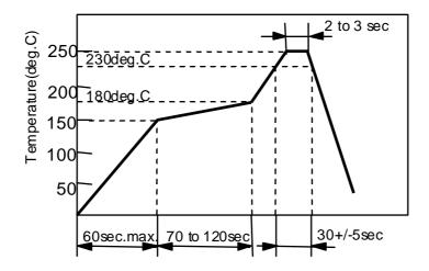
IR REFLOW SOLDERING
